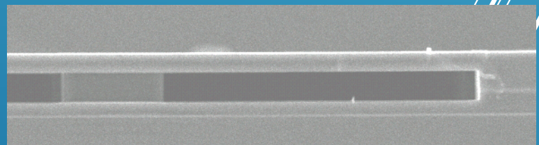
IceMOS embedded Cavity Feature
