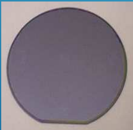
SOI Wafer with <1.5mm edge terrace
