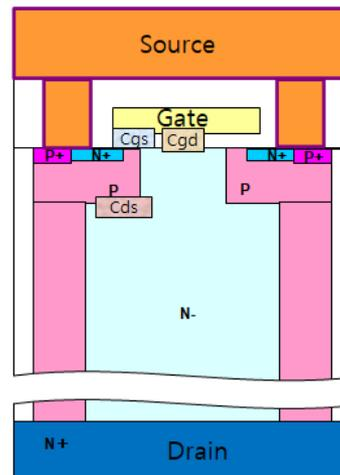
Fig19. Capacitance of the SJMOSFET structure
