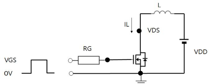
Fig.2 Example of UIS circuit
