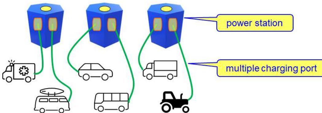
In stations that charge several electric vehicles simultaneously, it is necessary to connect 15kW~30kW charger units in parallel to output 100kW or more.
