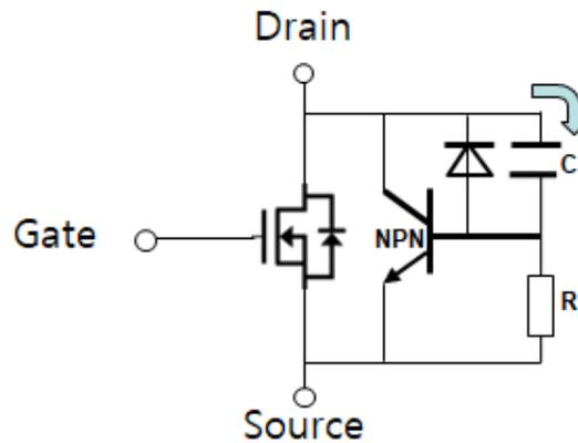
Fig.4 Equivalent Circuit
