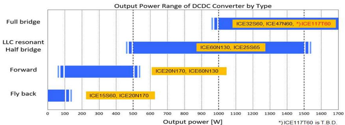
Circuit choice may be different depending on the output power. Full bridge may have over 1700W Power therefore please select the appropriate product depend on the power range. For example, the case of 100W Fly back , we offer ICE20N170 for Max Id=20A or ICE15S60 for Max Id=15A.
