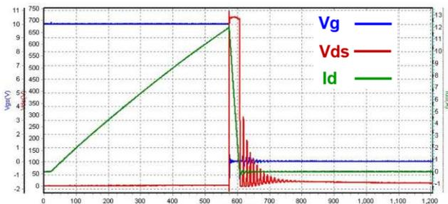
Fig. 1 output wave example of UIS test.
