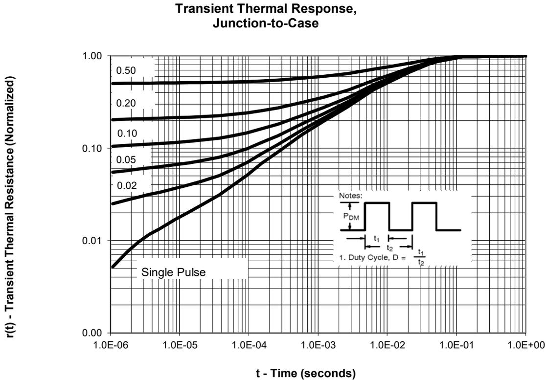
Fig.25 Transient Thermal Resistance  $r(t)$ -pulse width time
