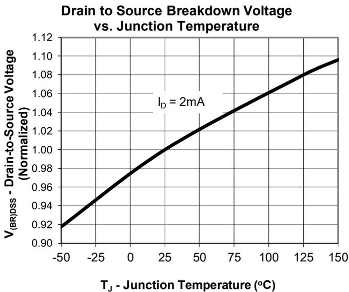
Fig.16  $V_{(BR)DSS}$  Vs  $T_J$  Junction temperature.
