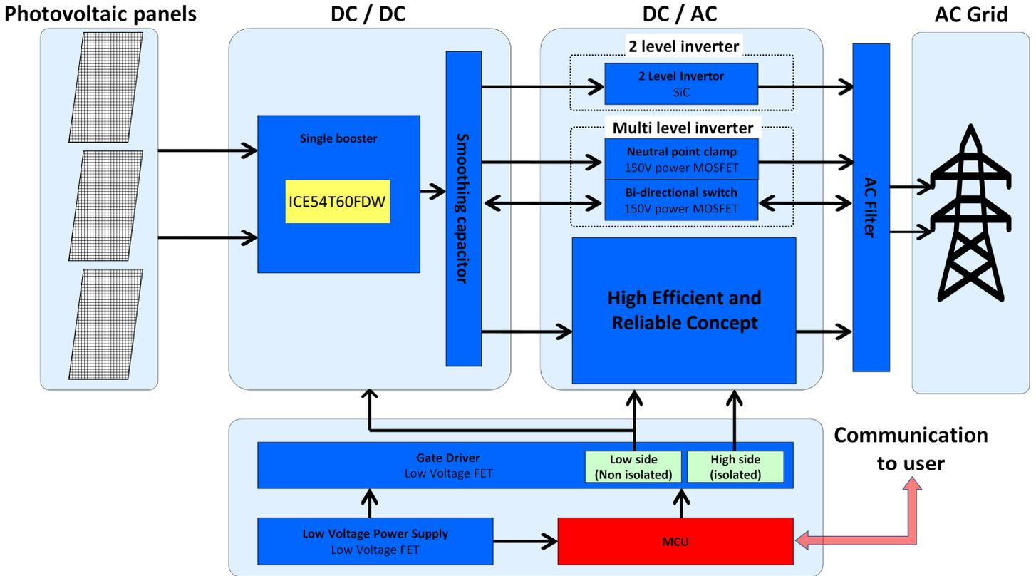
For DCDC, a single booster is usually used. and for DCAC, there are three methods for DCAC block.
