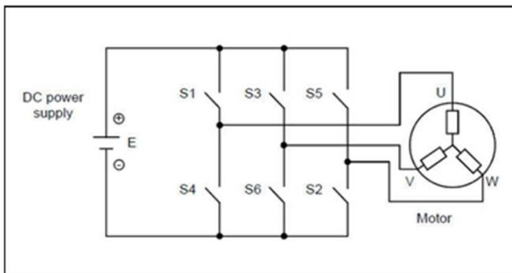
The topology is based on six power switches to supply voltage to a motor to control its speed, position or electromagnetic torque. Each half bridge operates in hard switching commutation on an ohmic-inductive load (motor) with a continuous load current and every commutation requires the freewheeling phase done by six diodes coupled with the power switches, to conduct reverse current.
