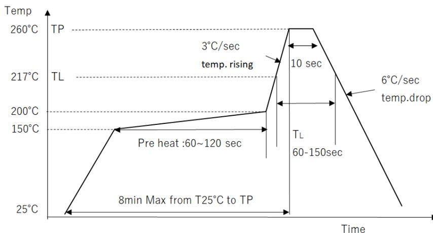
Fig.8 An Example of a Flow Temperature Profile.
