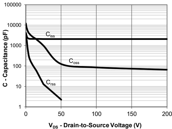
Fig. 18  $C_{iss}, C_{oss}, C_{rss}$  vs  $V_{DS}$
