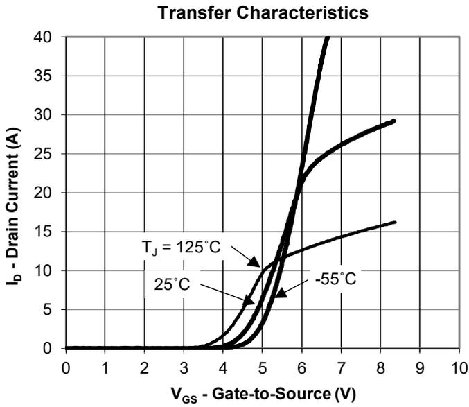
Fig 10  $V_{GS}$ - $I_{DS}$  Characteristic
