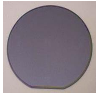
SOI Wafer with <1.5mm edge terrace
