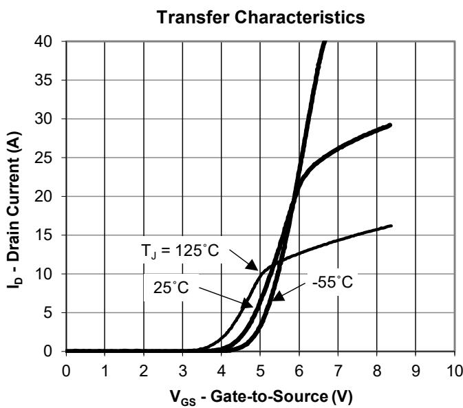
Fig 10  $V_{GS}$ - $I_D$  Characteristic
