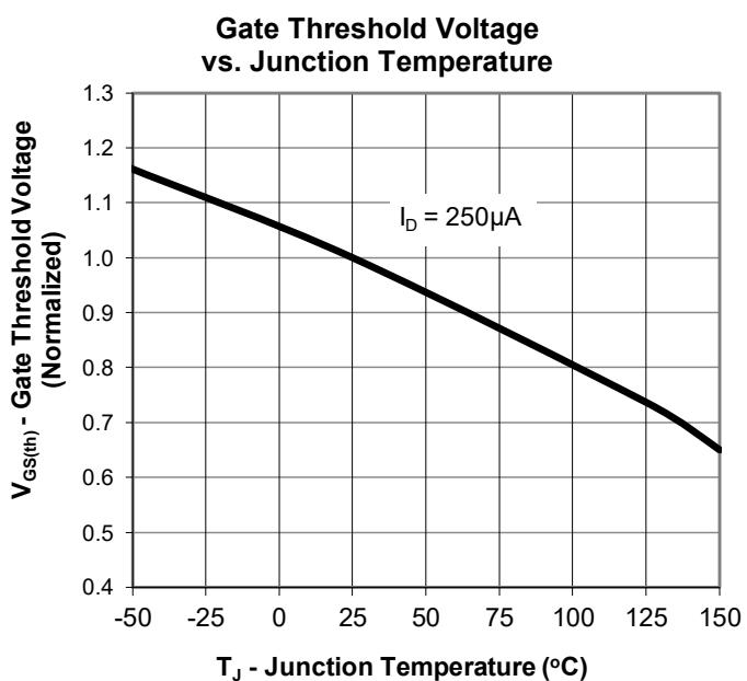
Fig.11  $V_{GS(th)}$  Vs  $T_J$  Junction temperature.
