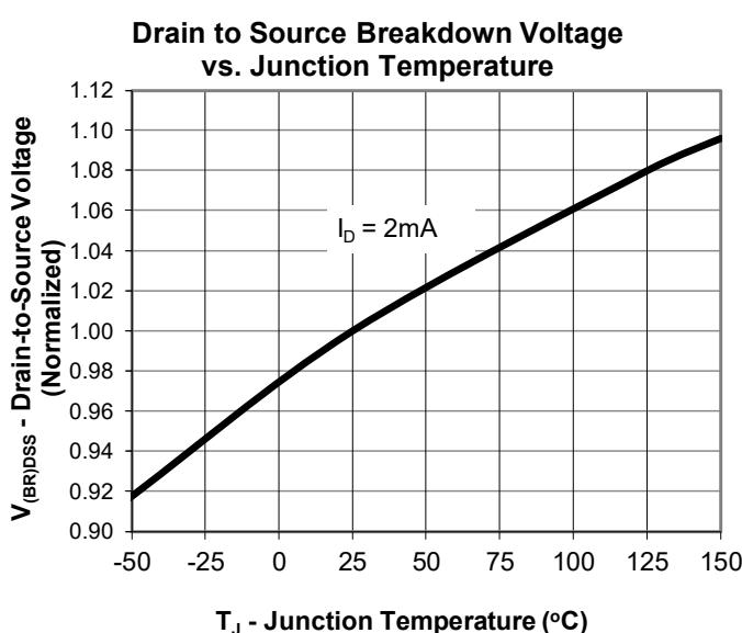
Fig.16  $V_{(BR)DSS}$  Vs  $T_j$  Junction temperature.
