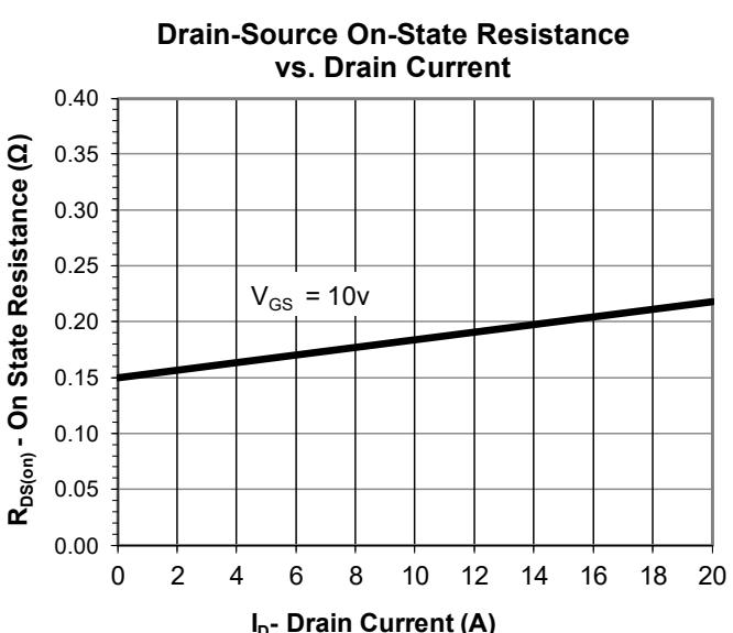
Fig.13  $I_D$  –  $R_{DS(ON)}$
