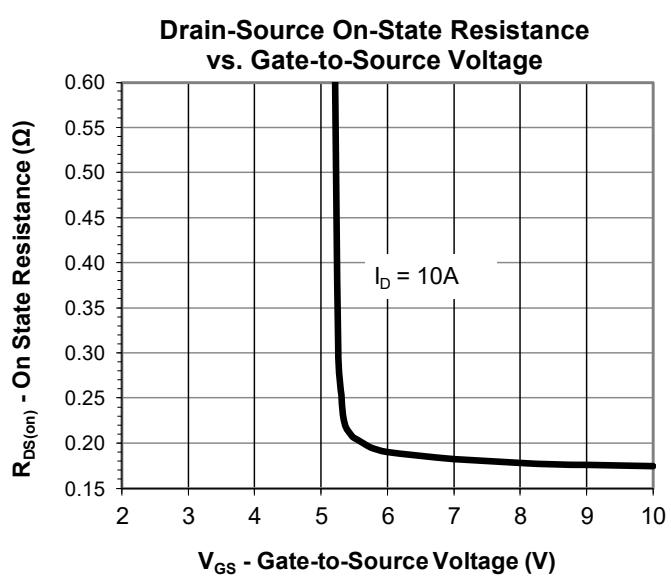
Fig.17  $V_{GS}$ -  $R_{DSON}$
