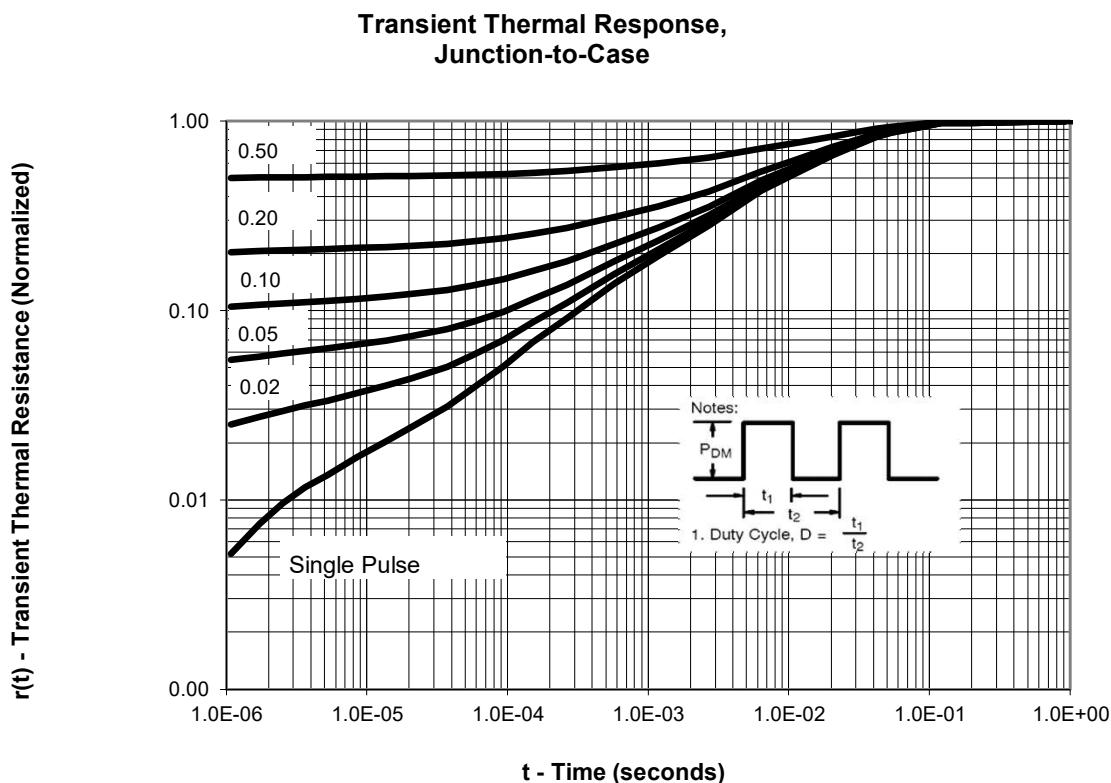
Fig.25 瞬态热阻  $r(t)$ -pulse width time
